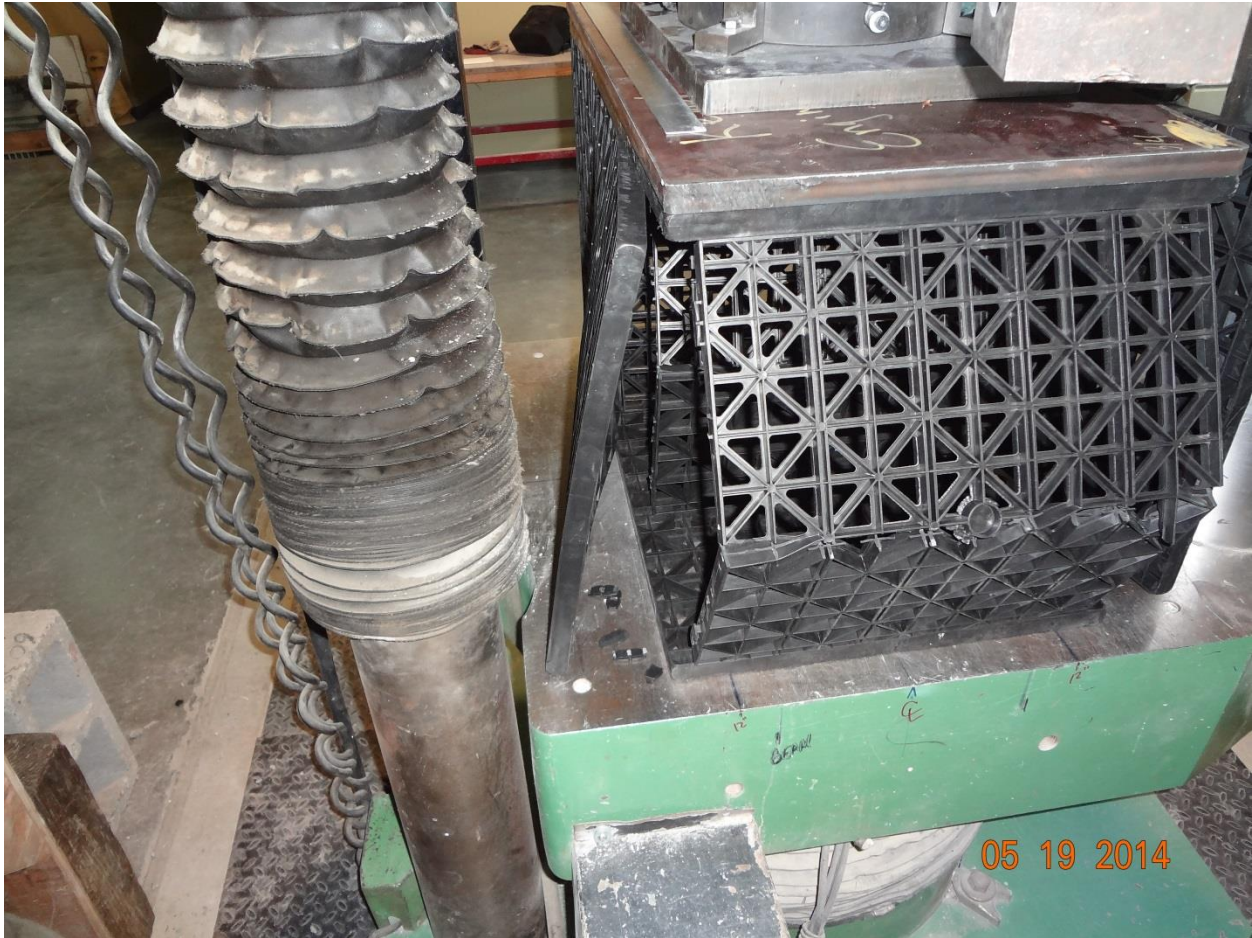
Figure 10: Second test block failure from the back side
