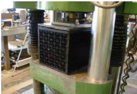
Ecology Block 6530B after Failure
