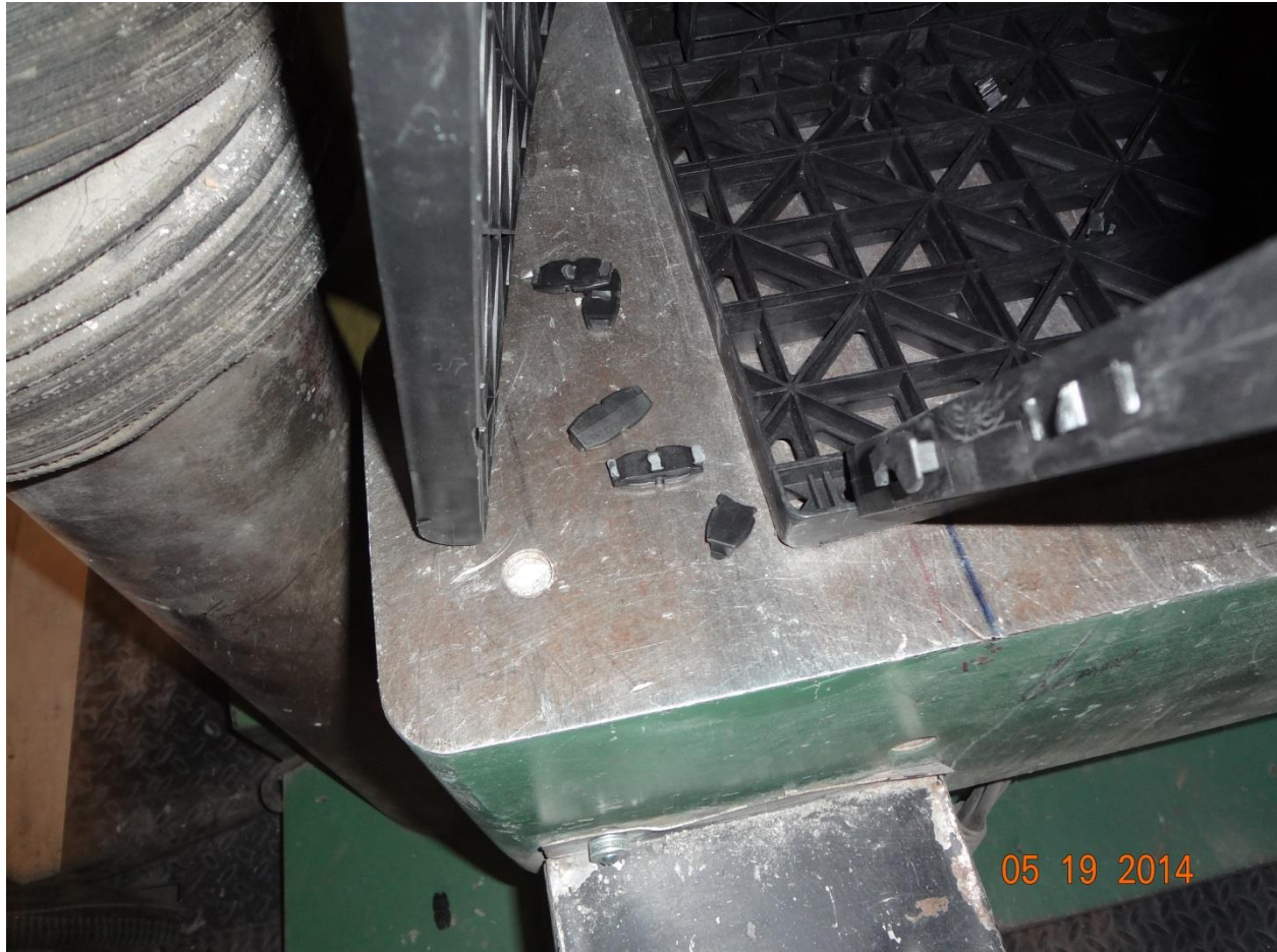
Figure 11: Broken Tabs from second test block
