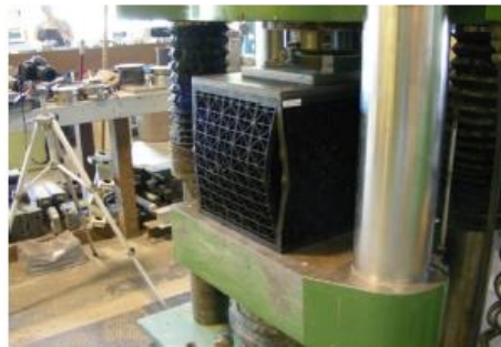
Ecology Block 6530C @ Failure
