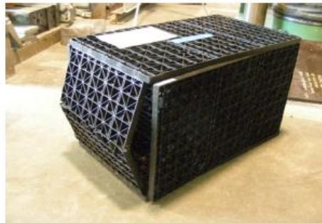
Ecology Block 6530C after Failure
