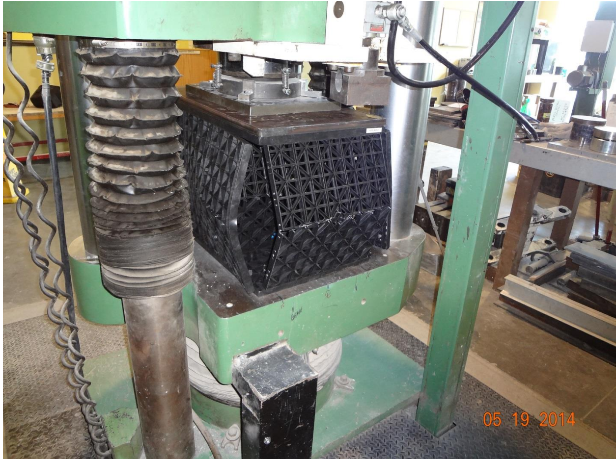
Figure 12: Third test block failure from backside
